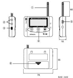
② Sensor Jack 3 POWER Button 4 Operation Buttons (DISPLAY INTERVAL
